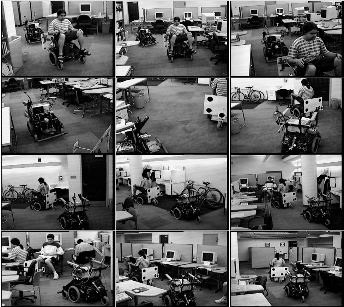
Figure 9: Twelve frames from a sequence that shows a completely autonomous mobile platform following a manually-driven platform around a cluster of tables. The temporal sequence of the frames corresponds to a row-major order.
